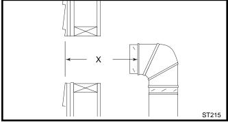
Fig. 27 Measure the horizontal length.
